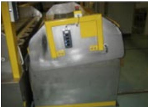
Figure 22: Slitter 13 before modification — risk of crushing fingers
