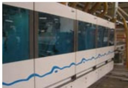
Figure 34: Some noisy machine tools are now in acoustic enclosures
