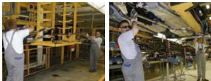
*Figures 3 and 4: Operators picking up the exhaust from the rack and decking it under the vehicle.*
