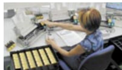
Figure 16: Insertion of the head into the printer (original layout)
