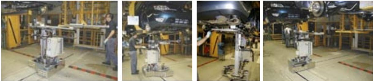
Figure 7: The manipulator carries the exhaust towards the car – Figure 8: The operator makes the manipulator lift the exhaust – Figure 9: The operator fixes the exhaust to the car – Figure 10: The manipulator goes towards the rack in order to pick up a new exhaust
