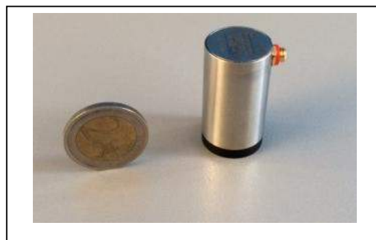
Fig. 2 – Sensore EA Vallen VS75-SIC
